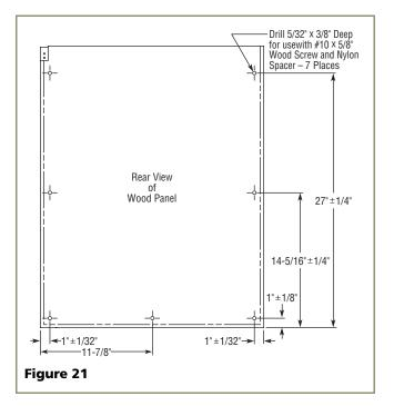
4. Attach the door panel to the overlay panel using #10 x 5/8" wood screws and nylon spacers. The nylon spacers fit between the overlay panel and the door panel as shown in **Figure 22**. The spacers allow the original door panel to slide back into the 1/4"-thick door reveal (channel).
